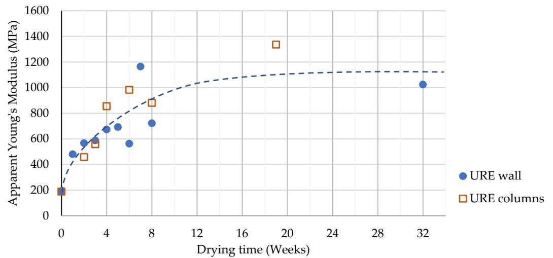
**Figure 9.** Evolution of Apparent Young's modulus of URE wall with drying time along with its tendency shown by dashed line. The results of wall are compared to the one of columns prepared by using similar soil and have similar dry density [16].
