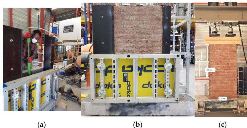
**Figure 4.** (a) Compaction of earth in a formwork using a pneumatic hammer. (b) Removing formwork after compaction, compacted earth layer can be observed. (c) URE wall subjected to mechanical test using two electric actuators.
