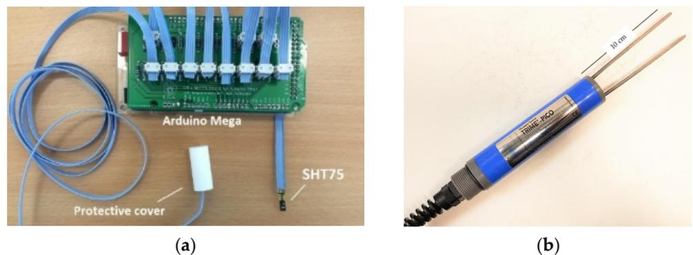
**Figure 6.** (a) Capacitive sensors, (b) Time Domaine Reflectometer.
