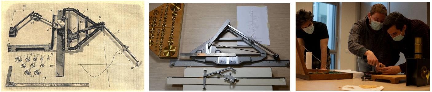
Figure 3. The Mader-Ott Harmonic Analyser used from 1909 to 1960. a) Illustration of how the harmonic analyser works b) Mader-Ott Harmonic Analyser from Optics department lab collection, FEMTO-ST Institute, Besançon. c) Master students from graduate school EIPHI during labwork with the harmonic analyser
