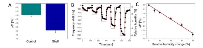
Figure 3. (A) Cantilever response towards a humidity change from 20 % to 60 % (error bars represent the standard error of the mean for n = 5); (B) Online measurements of the resonant frequency shift for increasing levels of humidity; (C) endpoint values of the relative humidity change as a function of the resonant frequency shift (error bars represent the standard error of the mean for n = 3)
