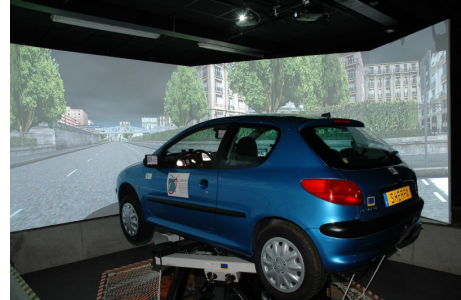
Fig. 6: SHERPA dynamic driving simulator.
