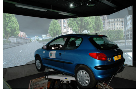
Fig. 6: SHERPA dynamic driving simulator.
