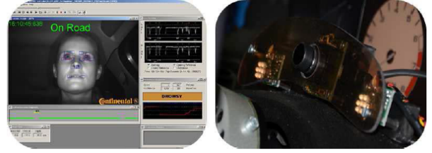
Fig. 4: Continental driver monitoring system.
