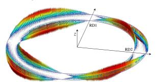
Fig. 3. Distribution of b in the air-gap between two stacked sheets
