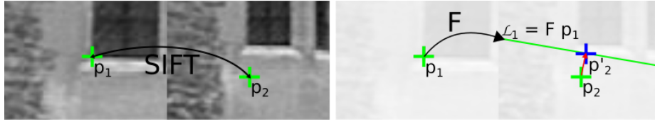
Fig. 2. From an imperfect match (p_1, p_2) considered inlier by AC-RanSaC, the “perfect match” (p_1, p'_2) is constructed using p'_2 the orthogonal projection of p_2 on the epipolar line \mathcal{L}_1 = F p_1 where F is a realistic fundamental matrix given by AC-RanSaC. This does not guarantee that p'_2 represents the same physical point as p_1 , but that some 3D point at possibly different depth projects exactly at p_1 and p'_2 . Figure originates from original paper [31]
