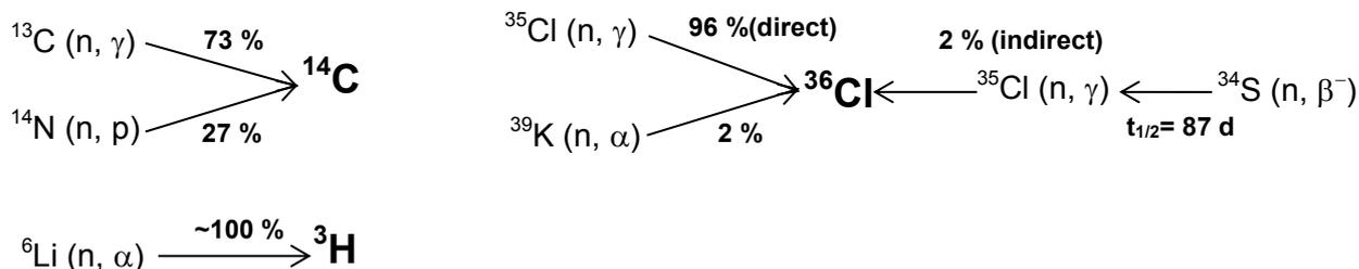
More generally, 144 i-radionuclides are found by the activation of 52 k-impurities through the proposed method. Therefore an output result of the method is the activation matrix  $M$  whose terms  $m_{ki}$  represent the contributions of the  $k$  impurities to  $i$  radionuclides at the scale of the whole pile. This activation matrix  $M$  is a key result to compare from a pile to another to assess the physical robustness of the method, a comparison work that is planned as a next step.
