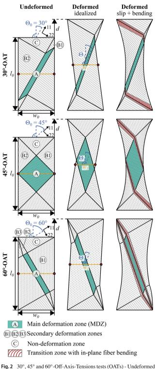
geometries, idealized deformed specimens and deformed specimens taking into account fiber slip and bending deformation in the transition zones
