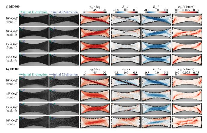
**Fig.8** Deformed specimens without (left) and without (second-left) dots as well as resulting strain distributions at an engineering strain of  $\varepsilon = 0.25$  during Off-Axis-Tension tests (OATs) for medium-sized specimens (320 x 160 mm) of (a) Biax-NCF and (b) UD-NCF
