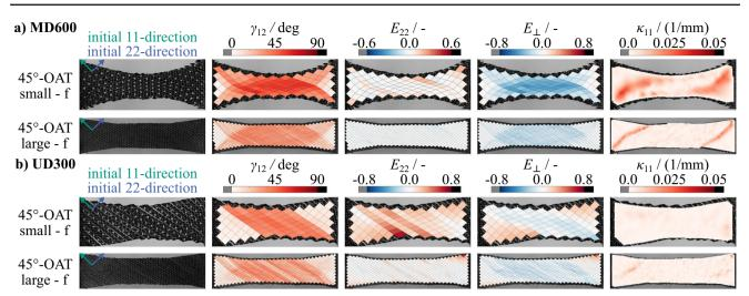
Fig. 13 Deformed specimens and strain distributions during Off-Axis-Tensions tests (OATs) (a) for Biax-NCF and (b) UD-NCF of different specimen sizes
