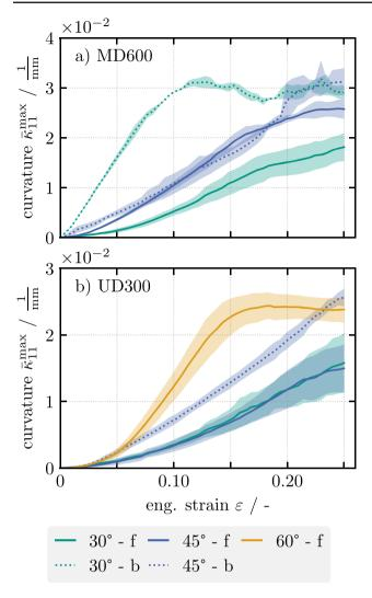
Fig. 10 Averaged curvature of the OATs for the a) Biax-NCF (MD600) and b) UD-NCF (UD300)
