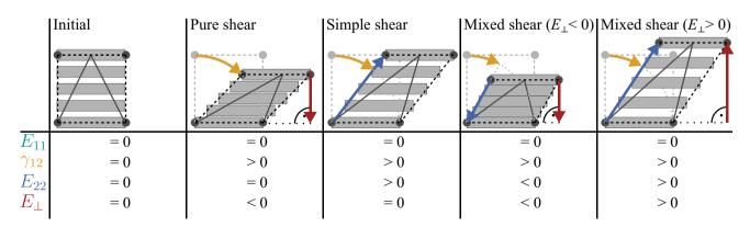
Fig. 4 Schematical representation of different deformation modes and the corresponding resulting strains
