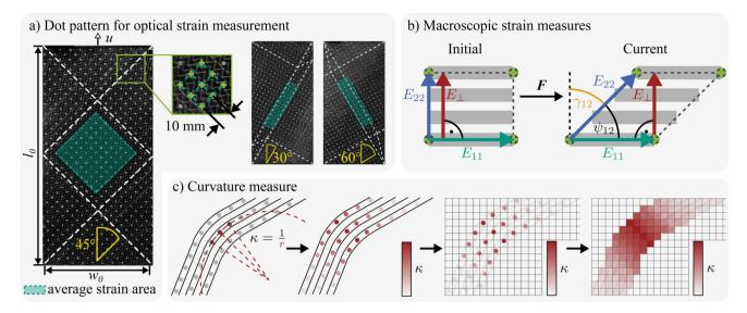
Fig. 3 (a) Dot pattern utilized during 2D-DIC to measure (b) macroscopic strains as well as (c) resulting curvature in fiber direction
