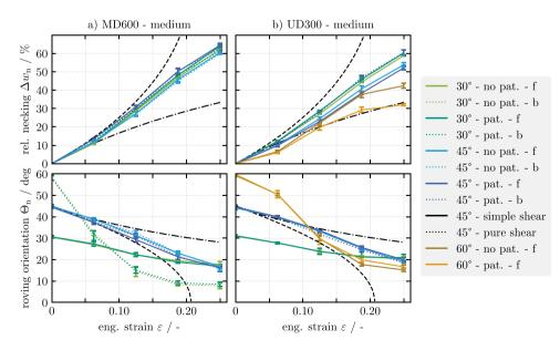
**Fig. 7** Relative necking  $\Delta w_n$  and roving orientation  $\Theta_n$  in the MDZ of the OATs for the (a) Biax-NCF and (b) UD-NCF for all tests with and without a dot pattern (pat.) on the front (f) or back (b) of the medium-sized specimens (320 x 160 mm)
