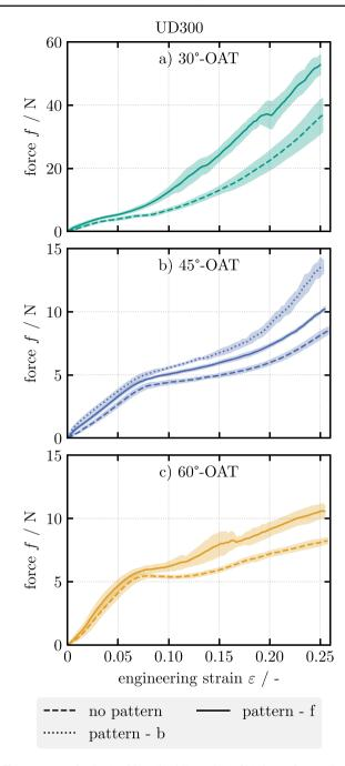
**Fig. 6** Forces in the (a)  $30^{\circ}$ -, (b)  $45^{\circ}$ - and (c)  $60^{\circ}$ -OATs for mediumsized specimens (320 x 160 mm) of the UD-NCF (UD300) with and without a dot pattern on the front (f) or the back (b)
