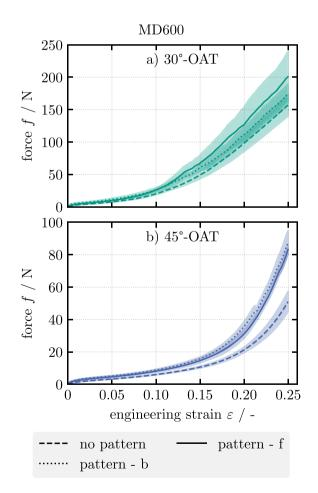
**Fig. 5** Forces in the (a)  $30^{\circ}$ - and (b)  $45^{\circ}$ -OATs for medium-sized specimens (320 x 160 mm) of the Biax-NCF (MD600) with and without a dot pattern on the front (f) or the back (b)
