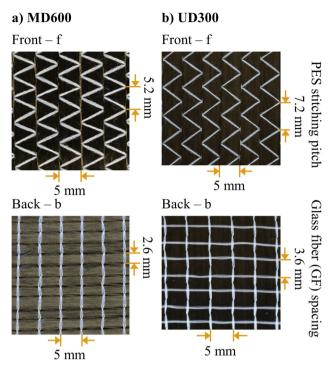
Fig. 1 (a) Bidirectional (0°/90°) NCF MD600 and (b) unidirectional NCF UD300 and
