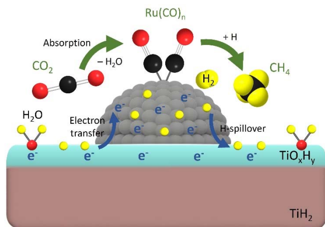
Scheme 1. Proposed relationship between structure, MSI and catalytic performances of m RTH towards \text{CO}_2 methanation.
