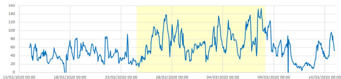
Figure 19b: O_3 levels measured by the second air monitoring micro - station, before, during and after a holiday period (based on daily averages).
