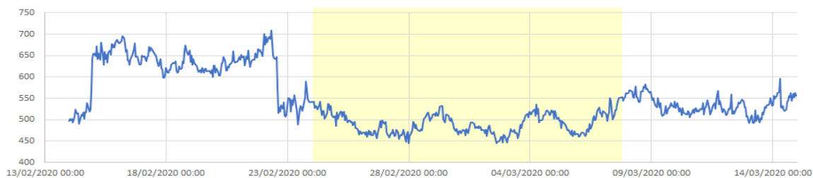
Figure 17b: CO 2 levels measured by a second air monitoring micro - station installed in a residential area near the school, before, during and after a holiday period (based on daily averages).
