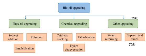
Fig. 5. Bio-oil upgrading methods.
