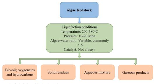
**Fig. 4.** Flowchart illustrating the hydrothermal liquefaction of algae. Adapted from Galadima and Muraza (2018).
