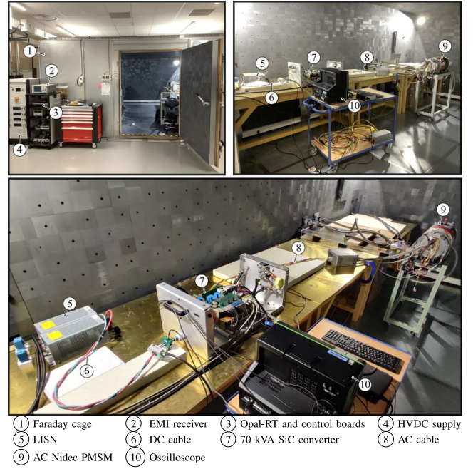
Fig. 12. Overview of the experimental setup for EMC tests.
