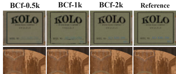
Figure 10: Effect of the resolution of the neural compressed features on the visual reconstruction. Note that this resolution parameter is directly linked to the compression ratio our method achieve.
