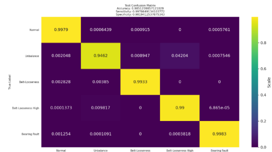
Fig. 9. Confusion matrix of the Neural Network based diagnostic model
