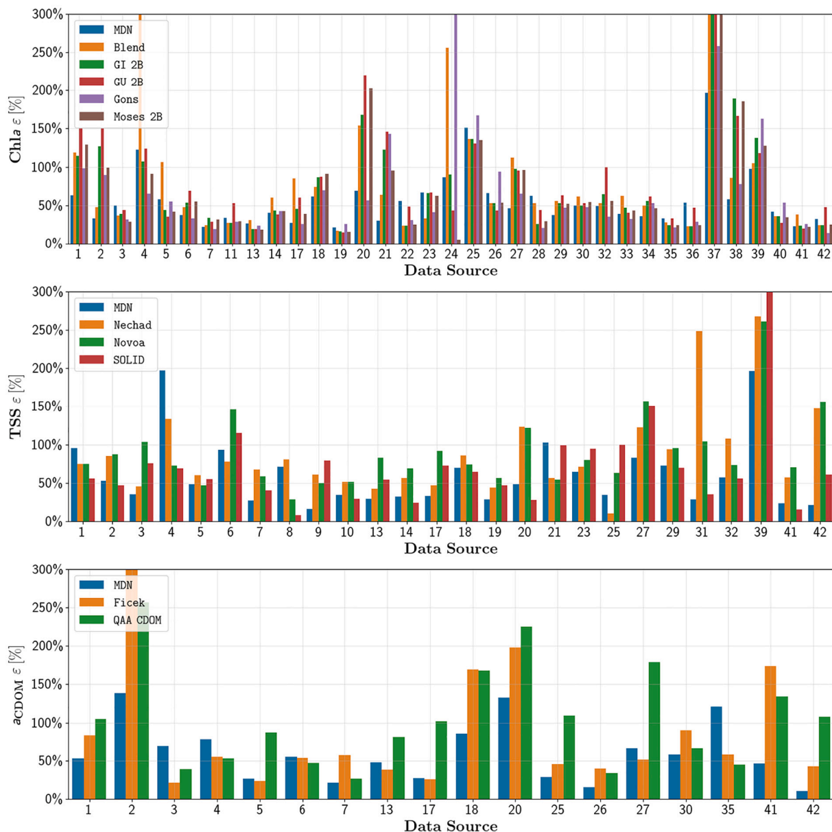
Fig. 5. Performance assessments based on the leave-one-out (LOO) experiments for an MSI-like mission for Chla, TSS, and a_{\text{cdom}}(440) . See Appendix A for more details on the data sources, indices, and corresponding average R_{rs} spectra (Figure A). Equations for the state-of-the-art algorithms are provided in Appendix C.
