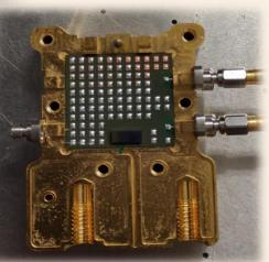
An active tunable noise source (NS) was developed in the 140 to 170 GHz (D-band) [7]. The extracted available excess noise ratios (ENR<sub>av</sub>) of the NS were ranged from 0 dB to 37 dB when wafer-level noise measurements were performed in D-band. While the ENR<sub>av</sub> values of the packaged NS were limited to 25 dB in the G-band, indicating a loss of ~12 dB in the packaged configuration.
