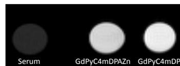
**Fig. 3.**  $T_1$ -weighted phantom images in mouse serum without or with 0.2 mM GdPyC4mDPA in the presence and in the absence of 1 eq. of  $\text{Zn}^{2+}$  (37 °C). Images were acquired at 9.4 T using spin echo sequence with TE = 16 ms, TR = 500 ms.
