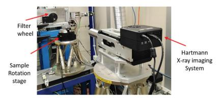
Figure 3. Picture of the experimental set-up installed at SYRMEP beamline of ELETTRA synchrotron illustrating the relative positions of the Hartmann X-ray imaging system and the sample rotation stage compared to the direction of the X-ray beam.
