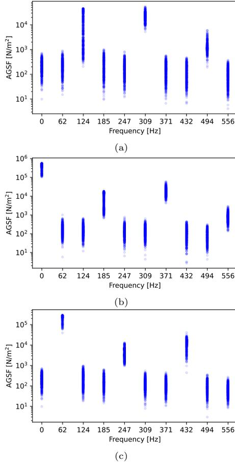
Figure 5: Air-gap surface force  $[\text{N}/\text{m}^2]$  samples generated for different spatial orders at  $\Omega = 463$  RPM for three different spatial orders (a) shows AGSF for  $r = -8$ , (b) for  $r = 0$  and (c) for  $r = +8$
