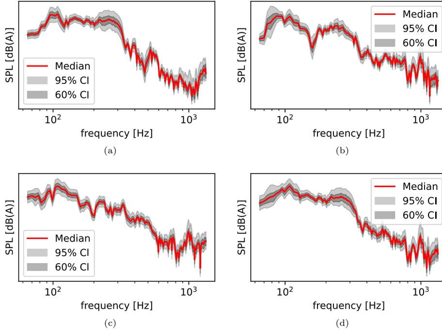
Figure 15: Interior SPL through left mount ( $M_1$ ) for a particular mechanical order  $k = 8$ . (a) Interior SPL contribution in  $x$  direction, (b) for  $y$  direction, (c) for  $z$  direction, and (d) shows the total contribution considering all three directions
