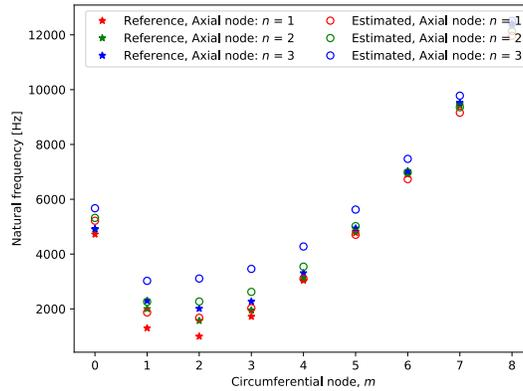
Figure 17: Comparison of natural frequencies of the stator system (design parameters same as the one used in [18], [page 117]) between the referenced data and the estimated data for different  $(m, n)$  pairs
