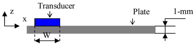
Figure 3. Description of 2D problem geometry
