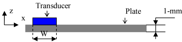
Figure 3. Description of 2D problem geometry
