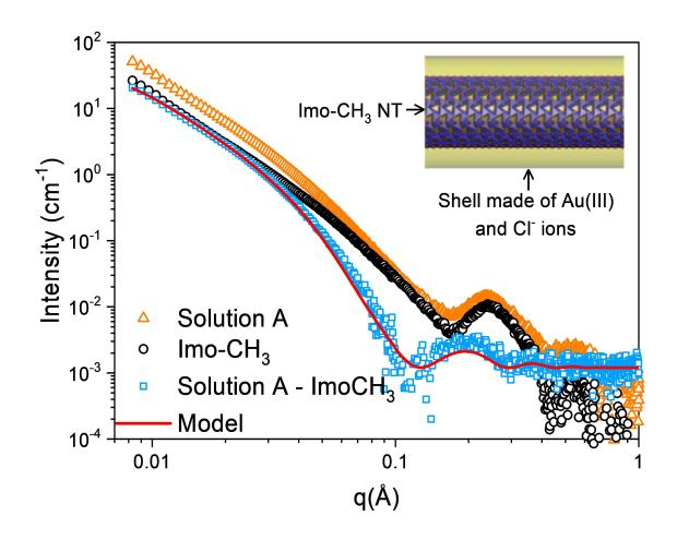
**Figure 1.** SAXS profile of Solution-A (orange triangles), pristine imogolite (black circles) and Solution-A after subtraction of pristine Imo-CH<sub>3</sub> scattering contribution (blue squares). The simulated SAXS profile for hollow cylinders made of surface adsorbed Au(III) and Cl<sup>-</sup> ions plus their fractal organization is also shown (red line curve) (see SI for details).
