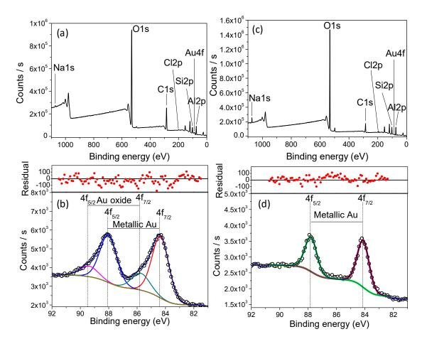
*Figure 4. XPS survey and Au 4f photoelectron core-level spectra of GNPs attached to Imo-CH*<sup>3</sup> *NTs prepared by UV photolysis (a,b) and gamma radiolysis (c,d).*
