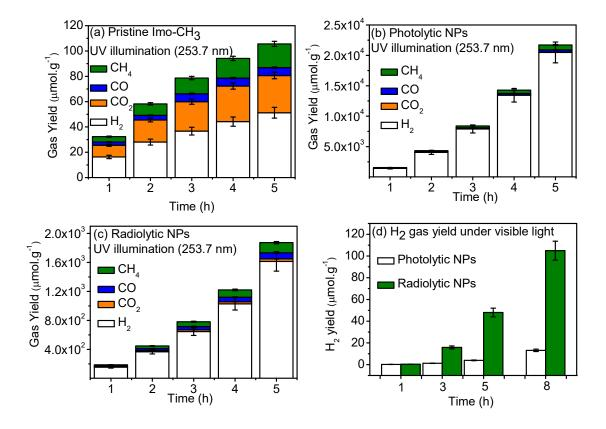
**Figure 5.** Gases produced as a function of UV illumination time for aqueous solutions of pristine (a) and GNP-coupled Imo-CH<sub>3</sub> NTs prepared by photolytic (b) and radiolytic (c) routes.  $H_2$  yield produced during visible light illumination of aqueous solutions of GNP-coupled Imo-CH<sub>3</sub> NTs (d).
