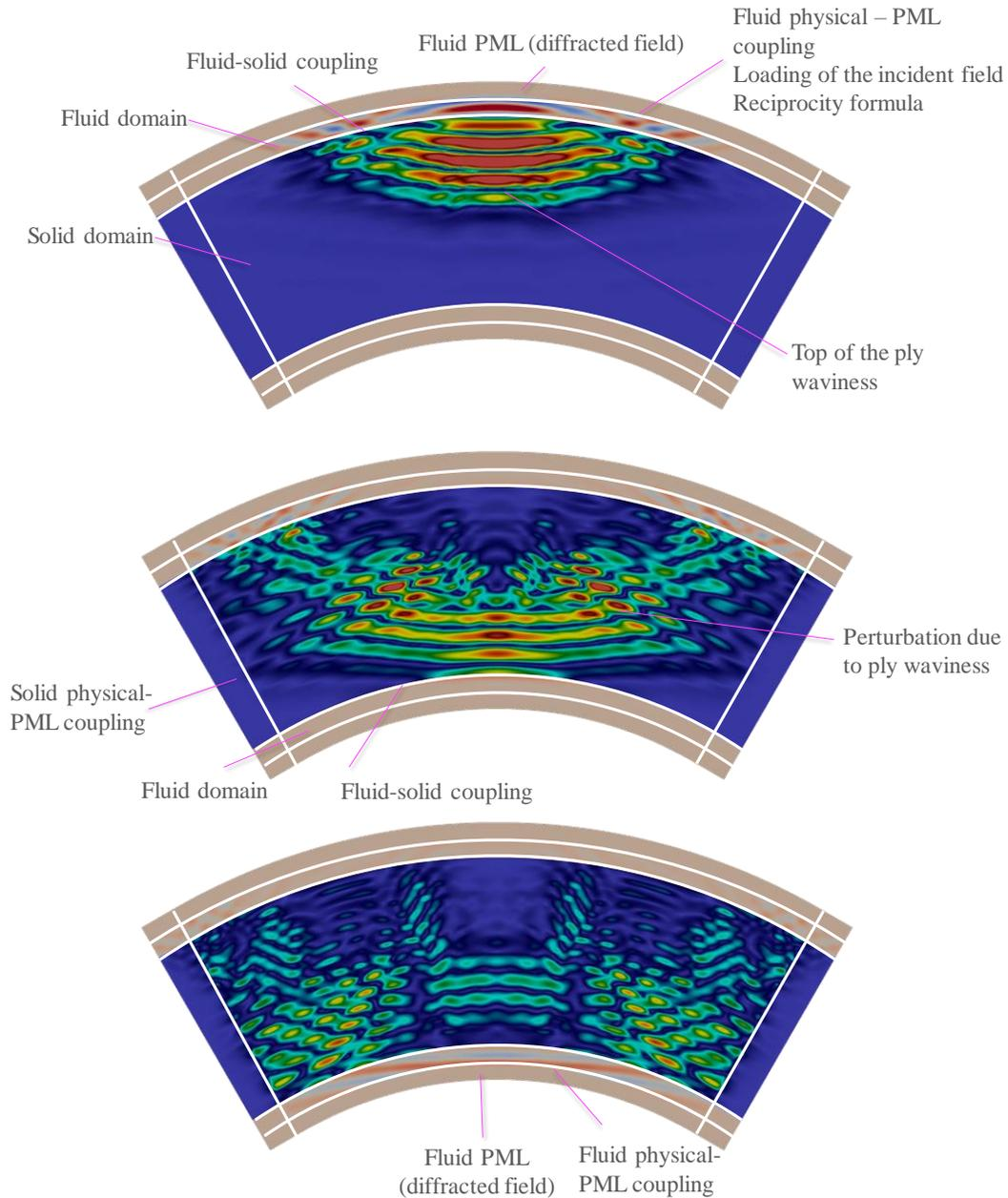
**FIGURE 10.** Snapshots of the SEM solution. In white lines are the edges of the macro-elements. The color corresponds to the magnitude of the displacement field (solid subdomains) or the pressure field (fluid subdomains).
