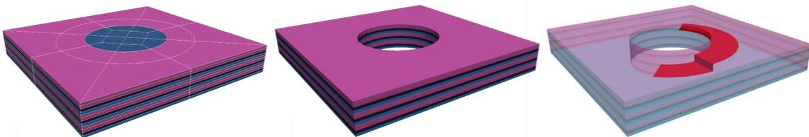
**FIGURE 6.** Example of macro-meshing pattern (left) whose centered macro-elements are eliminated to represent a borehole (center) and some mortar elements are eliminated to consider delamination and crack (in red on the right).
