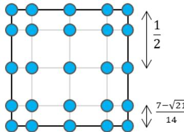
**FIGURE 4.** 4<sup>th</sup> order Gauss-Lobatto points on the unit quadrilateral.
