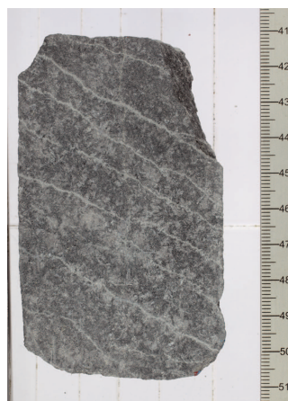
Figure F18. Closely spaced parallel veinlets at the top of the basaltic sill interval just below the chilled margin adjacent to the overlying sedimentary rock (385-U1550B-23X-1, 41–52 cm; 172.6 mbsf). Scale = cm.
