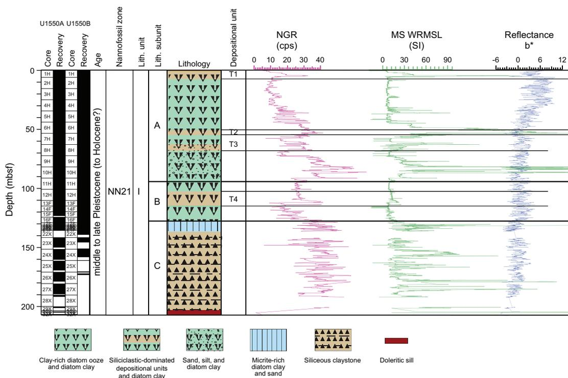
**Figure F4.** Lithostratigraphic column, Site U1550. Data on right are from Hole U1550A. Depth of the upper sill/sediment contact corresponds to Hole U1550A. NGR = natural gamma radiation, cps = counts per second, MS = magnetic susceptibility, WRMSL = Whole-Round Multisensor Logger.
