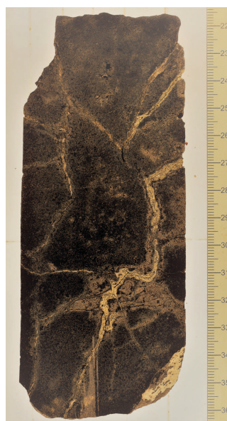
Figure F26. Irregular vein network filled with as many as four different materials (385-U1547B-45X-1, 23–36 cm).
