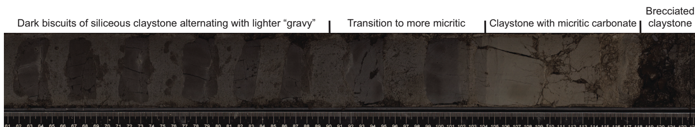
Figure F12. Typical lithologies and coring deformation (biscuiting) in Subunit ID (385-U1545A-75X-5, 61–123 cm).
