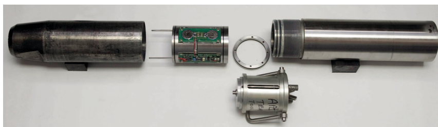
Figure F34. APCT-3 tool shoe (left) has a pocket to accept electronics, memory board, and battery (right) for temperature measurements while taking an APC core.
