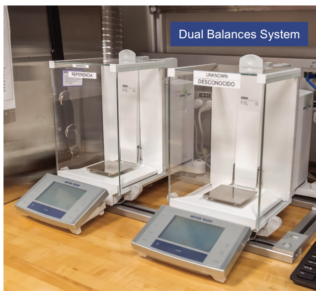
Figure F29. Dual balance system for wet and dry mass measurements.
