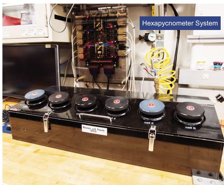
Figure F30. Hexapycnometer system for volume measurements.
