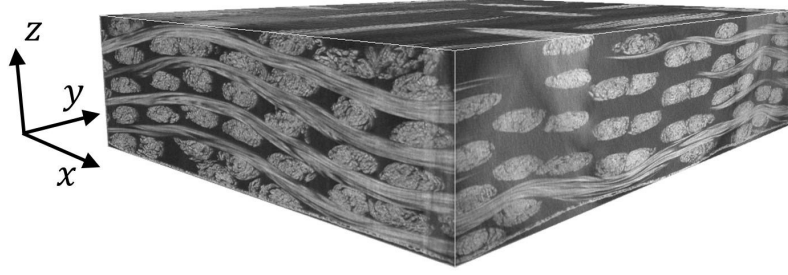
Figure 1: Reconstructed volume of the 3D woven fabric specimen.
