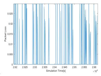
Fig. 5. URLLC packet loss illustration for reactive resource allocation.
