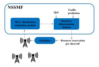
Fig. 1. Integration of the proposed resource dimensioning module.
