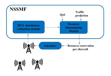
Fig. 6. Proposed architecture for the dimensioning framework.
