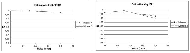
Figure 6 : Cosines of the Spectral Angles between real endmembers spectra and endmembers spectra estimated by N-FINDR and ICE algorithms for two different mixtures of four components
