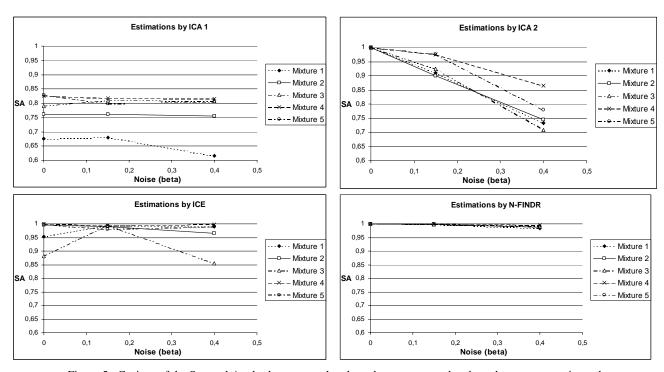
Figure 5 : Cosines of the Spectral Angles between real endmembers spectra and endmembers spectra estimated by the four algorithms for five different mixtures of three components
