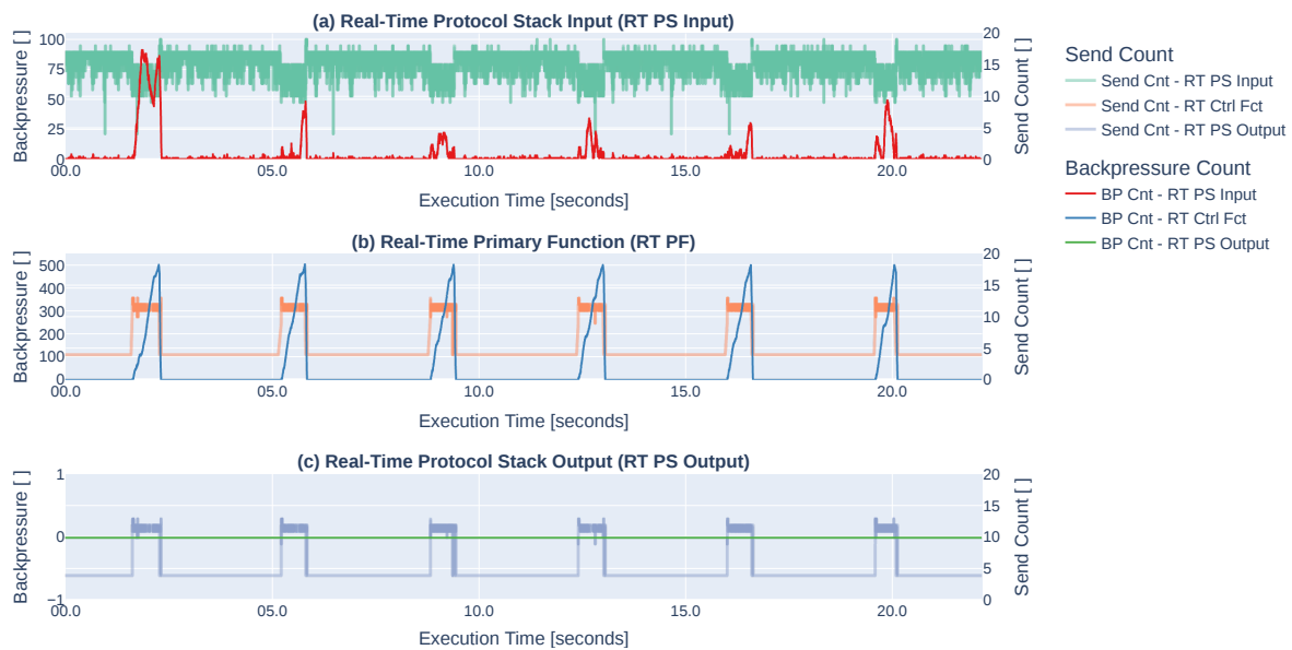
Figure 23. Timeseries diagram showing the periodic adaptation of the routing algorithm to cope with message bursts.
