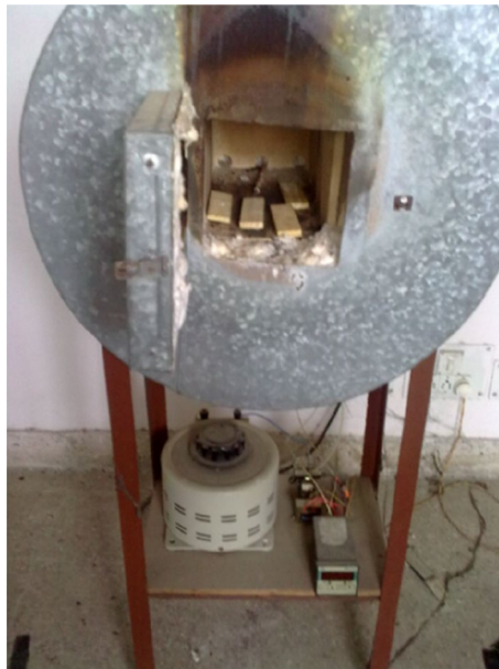
Fig. 2 A muffle furnace for heat treatment of wood adherent specimens
