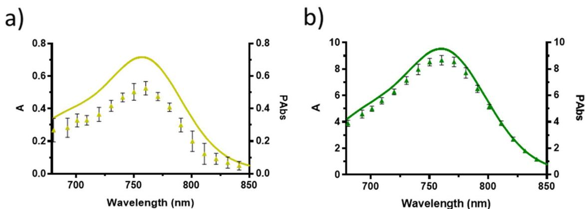
**Figure 2. Absorption spectra (continuous line) and PES (triangle) for nanoparticles batch. (a) NP-2.5% (yellow), (b) NP-50% (green). Laser fluence  $0.98 \text{ mJ}.\text{cm}^{-2}$ . The error bars for the PES corresponds to the median value  $\pm$  MAD. Absorbance values were corrected from dilution factor: no dilution for NP-2.5% and 10 times dilution for NP-50%. PAbs values were corrected from dilution factor: no dilution for NP-2.5% and three times dilution for NP-50%.**
