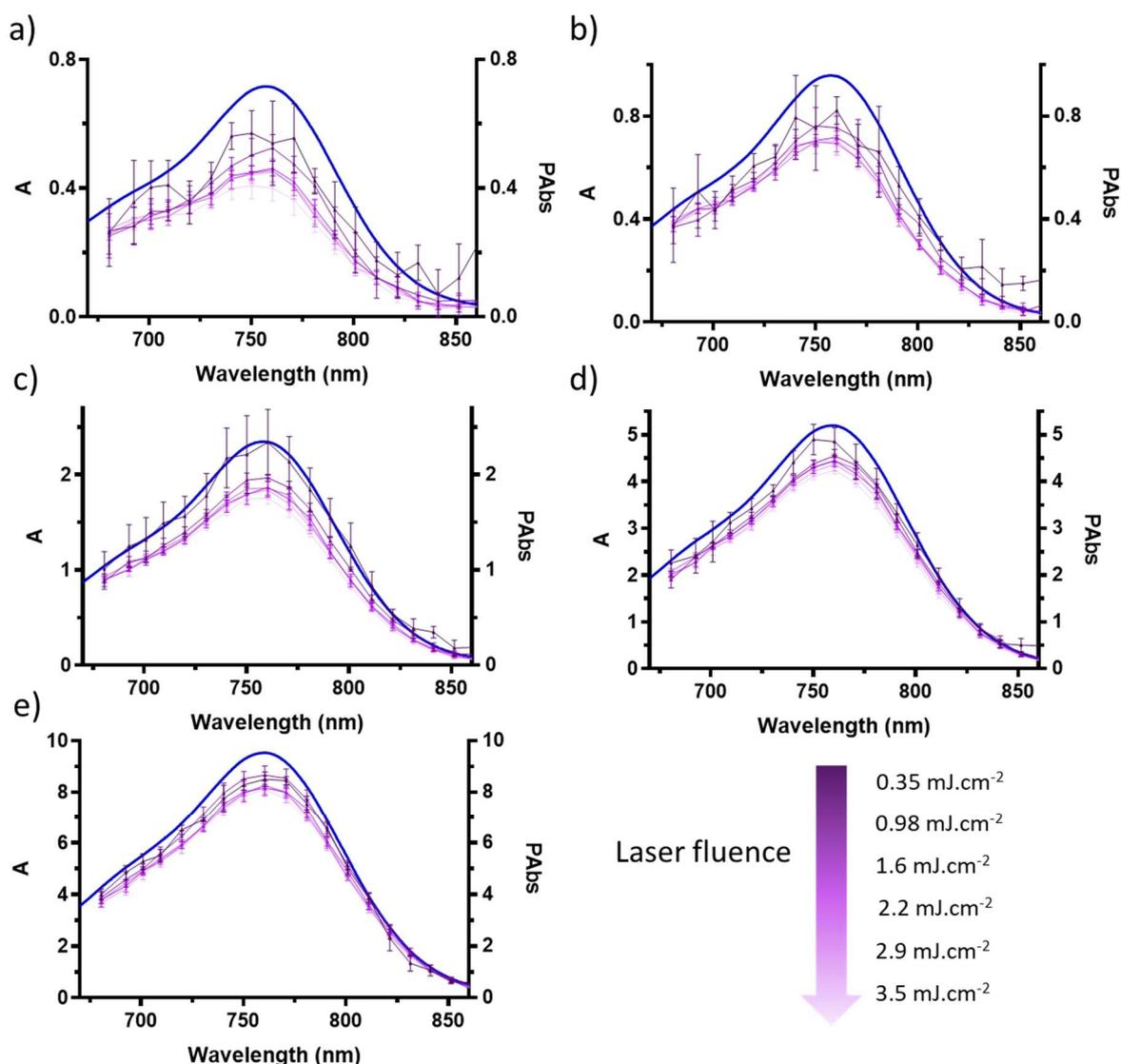
**Figure 5: Absorption spectra (continuous line) and PES (dots) of Bodipy NP for different laser fluences. (a) NP-2.5%, (b) NP-5%, (c) NP-10%, (d) NP-25%, (e) NP-50%. From dark to light violet respectively  $0.35 \text{ mJ.cm}^{-2}$ ,  $0.98 \text{ mJ.cm}^{-2}$  and  $1.6 \text{ mJ.cm}^{-2}$ ,  $2.2 \text{ mJ.cm}^{-2}$ ,  $2.9 \text{ mJ.cm}^{-2}$ ,  $3.5 \text{ mJ.cm}^{-2}$ . The arrow indicates the laser fluence increase. The error bars for the PES corresponds to the median value  $\pm$  MAD.**
