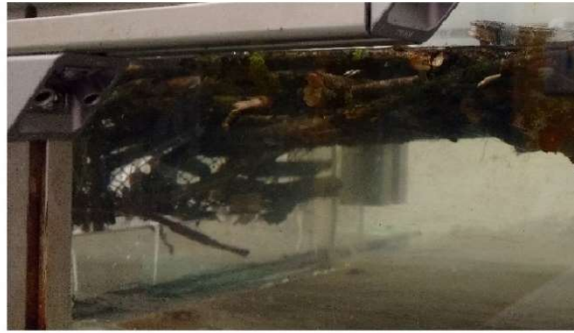
85 Figure 3: The logs accumulation upstream the barrier consists of a plug along the barrier and a floating carpet which are schematically defined, for the purpose of this study, by their height and length: ( h_p , L_p ) and ( h_c , L_c ) respectively. Example of logs accumulation upstream a flexible barrier exhibiting a long carpet (experiments presented in Piton et al. 2023).
