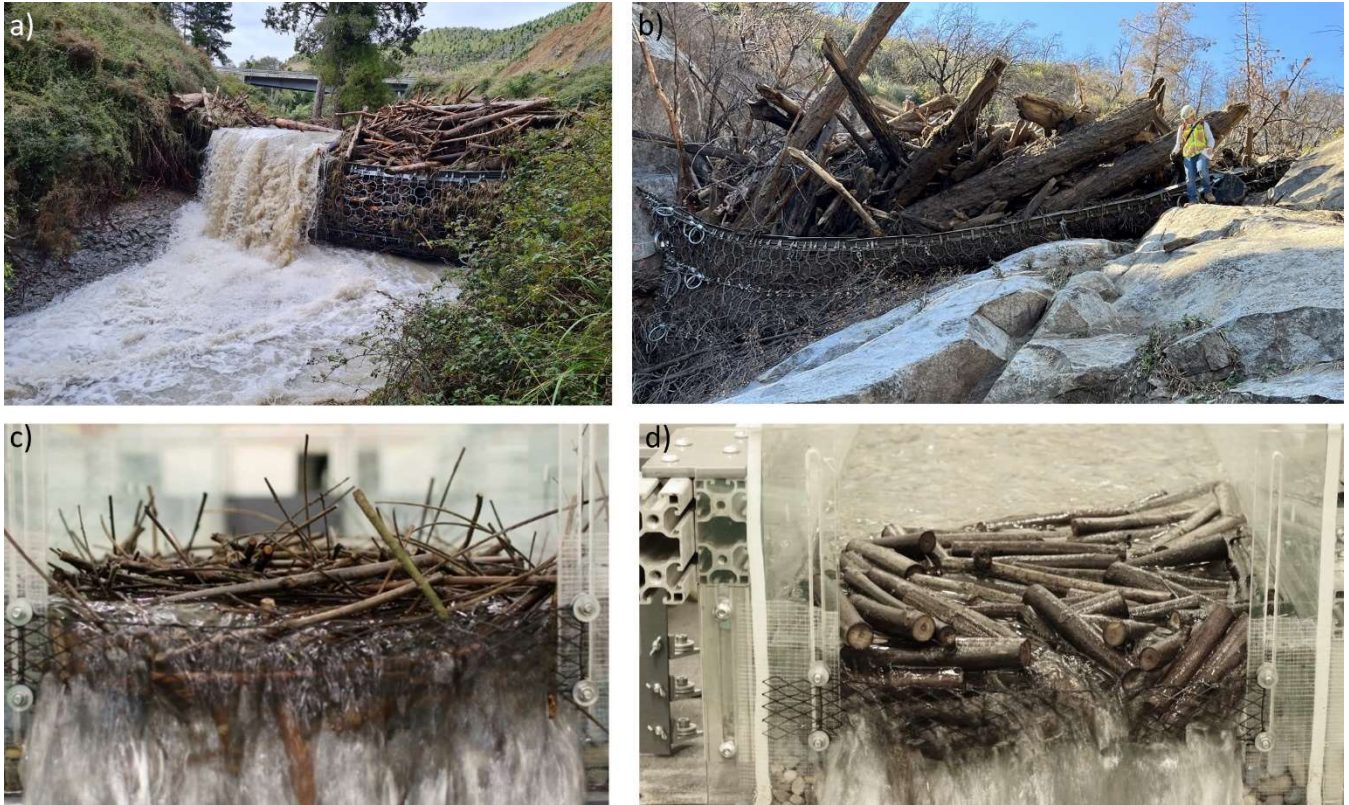
60 Figure 2: Woody debris trapped in flexible barriers in New Zealand (a) and in the USA (b) (Courtesy of Geobrugg and KANE GeoTech Inc respectively) and in the preliminary flume experiments with a smaller net with thin logs (c) and thick logs (d)
