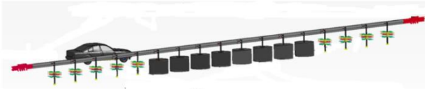
Figure 2 Simplified FE crashing model of VRS
