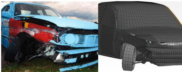
Figure 11 Vehicle after crash tests [14] and numerical model
