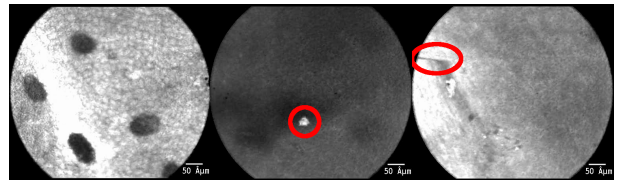
Fig. 1. Sample images acquired by a CellVizio endomicroscopy probe on a ficus benjamina leaf. Left : good contact conditions. Middle : Bad contact conditions. Right : motion artifact (circle) induced by local accelerations. Note how the middle image is dominated by noise, with artifacts from the fiber bundle showing up (circle).
