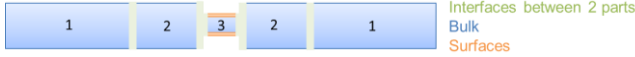
Figure 3. 2-D Areas and interfaces of the MNM device shown schematically (see Figure 1). Zone 1: Global resistance in the external branches (1). Zone 2: Total resistance within the connected microchannels (2). Zone 3: The two interfacial resistances and the nanoslit domain are assimilated to an ionic filter equivalent to the overall resistance in the nanoslit (3) (from 1 to 2 and 2 to 3).
