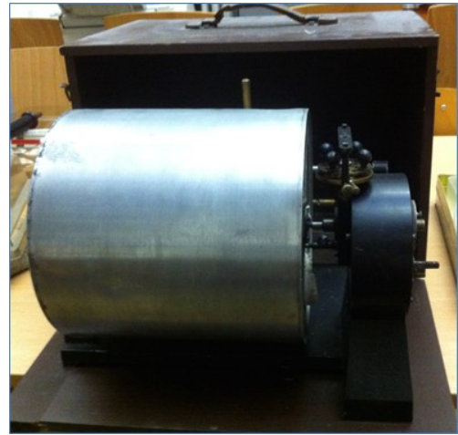
Figure 2: Gauthier portable Kymograph and its travel box.
