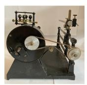
Figure 9: Belt, rolling disks, and drive bar.
