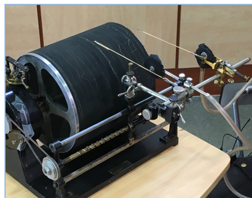
Figure 11: Complete Kymograph with 2 Marey's drums, straws and pen on blackened paper.
