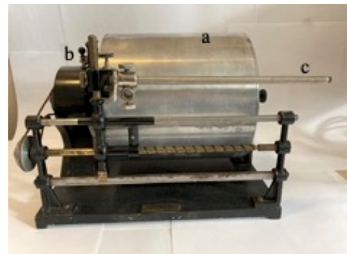
Figure 3: Gauthier Kymograph parts: a) drum, b) Foucault regulator, c) drive bar.
