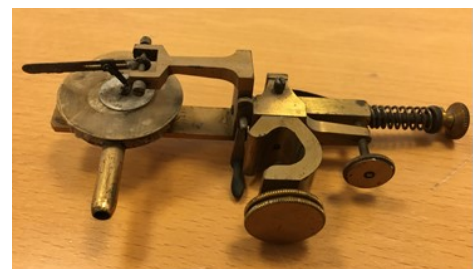
Figure 7: Marey's drum built by Verdin used with our kymograph.
