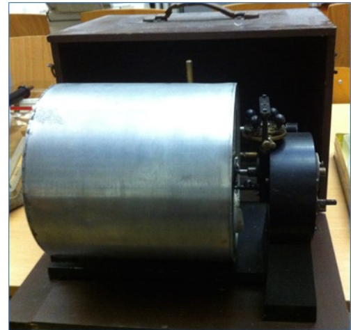
Figure 2: Gauthier portable Kymograph and its travel box.
