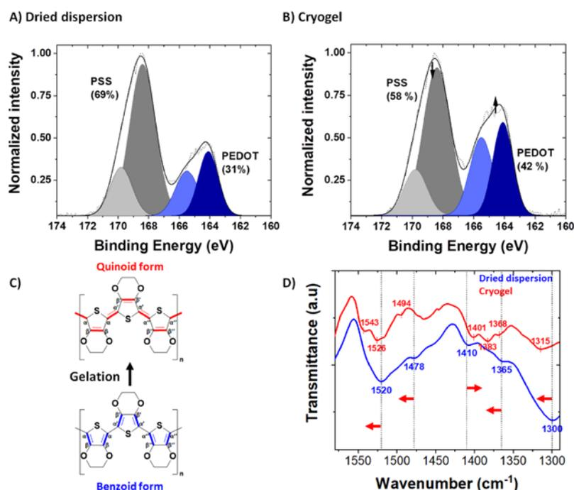
Figure 3 : A) S<sub>2p</sub> XPS spectrum of the dried PEDOT:PSS dispersion (self-supported drop casted film); B) S<sub>2p</sub> XPS spectrum of the quenched cryogel. (The molar % ratio is obtained via peak integration in grey for the PSS and blue for the PEDOT; gelation reduced the PSS
