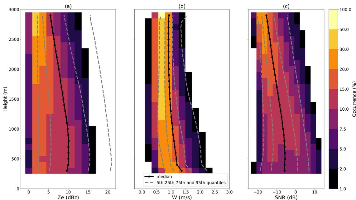
**Figure 4.** Median (black solid dotted line) and 5th, 25th, 75th and 95th quantiles (gray dashed lines) of the equivalent reflectivity  $Z_e$  (fig. 3a), the mean Doppler velocity  $W$  (fig. 3b) and the signal-to-noise ratio SNR (fig. 3c). The shading represents the occurrence along each radar gate (left blank below 1%). Pay attention to the non-linear colorbar.
