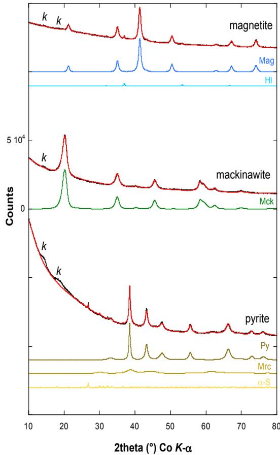
**Figure S1.** Rietveld refinement of XRD powder patterns of the magnetite, mackinawite and pyrite synthetic substrates prepared and used this study. Refined parameters values are reported in Table S1. Mag : magnetite ; HI : halite ; Mck : mackinawite ; Py : pyrite ; Mrc : marcasite ;  $\alpha$ -S, orthorhombic elemental sulfur; k : Kapton® window of the anoxic sample chamber.
