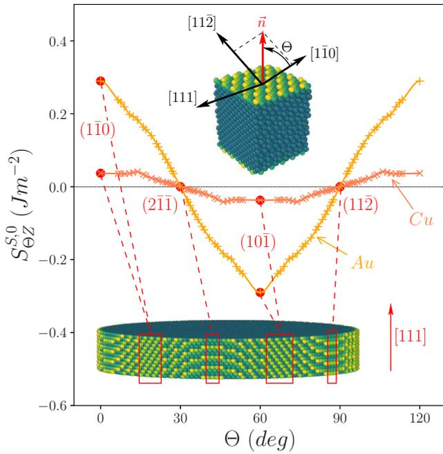
FIG. 2. Plot, as a function of  $\Theta$ , of the surface parameter  $S_{\Theta Z}^{S,0}$ , introduced in Eq. (4) and calculated from MS simulations using the SMA potential, on various Au and Cu slabs presenting different vicinal surfaces ( $hkl$ ) and sharing the same [111] direction corresponding to the nanowire axis. As an example, the case of a slab with  $(4\bar{1}\bar{3})$  surfaces corresponding to a value of  $\Theta \approx 46.1^\circ$  is shown.
