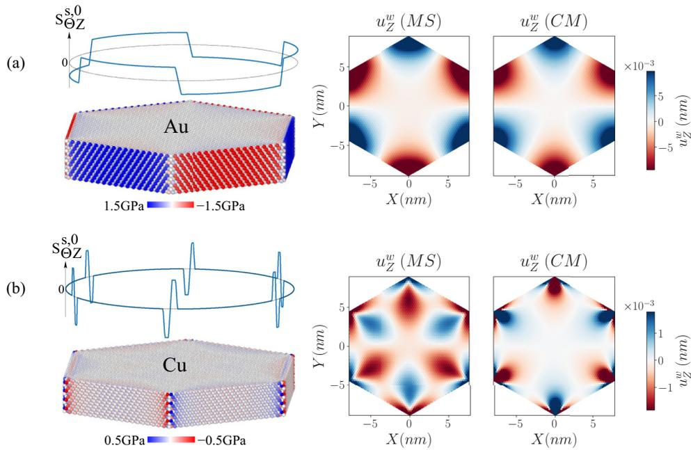
FIG. 4. Warp displacement fields  $u_Z^w$  (nanometers) in  $\langle 111 \rangle$  (a) Au and (b) Cu nanowires of hexagonal cross section with  $\{110\}$  surfaces. Comparison of the warp  $u_Z^w$  (MS) with  $u_Z^w$  (CM) predicted by Eq. (15) where the  $c_N$  are determined from the Fourier analysis of two different  $S_{\Theta Z}^{s,0}$  functions chosen to roughly reproduce the variations in atomic  $S_{\Theta Z}$  observed on the two simulated wire slices (see text).
