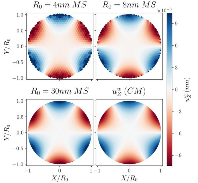
FIG. 3. Warp displacement fields  $u_Z^w$  (nanometers) in  $\langle 111 \rangle$  Au nanowires of circular cross section (for different radii:  $R_0 = 4, 8,$  and  $30$  nm). Comparison of the warp  $u_Z^w$ (MS) observed in the atomistic simulations with  $u_Z^w$ (CM) predicted by the continuum model in Eq. (15) where the  $c_N$  ( $1 \leq N \leq 48$ ) are determined from the Fourier analysis of  $S_{\Theta Z}^{S,0}$  shown in Fig. 2.
