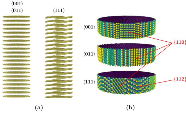
FIG. 1. (a) Illustration of the warp existing in  $\langle 111 \rangle$  (but not in  $\langle 001 \rangle$  or  $\langle 011 \rangle$ ) fcc nanowires. (b) Representation of the surfaces bounding these circular cross-section wires; only slices are shown here.
