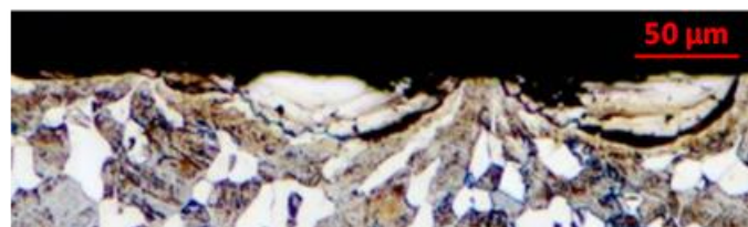
Fig. 12: Optical image of TTS island on the cross-section of a contact tested at a contact pressure of 300 MPa at 1000 fretting cycles.
