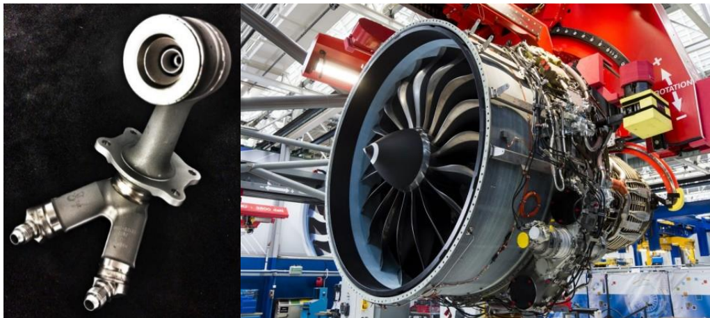
Figure 2-46 3D printed fuel nozzle, and the LEAP 1A engine [150]
