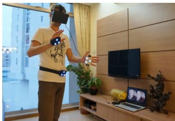
Figure 2-1 iMotion is a motion controller that creates haptic feedback by hand-and-arm interactions through a “virtual touchscreen” [35]
