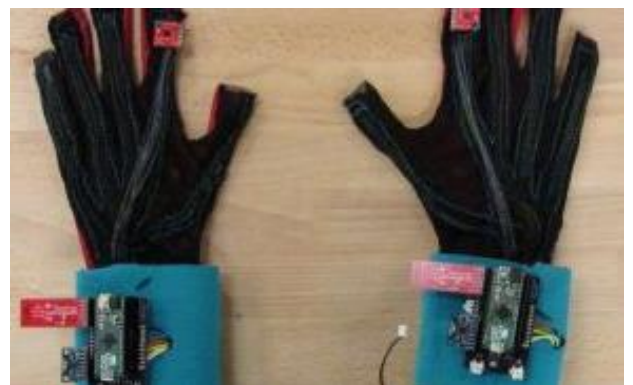
Figure 4-2 The special gloves designed to translate sign language into text or speech [264]
