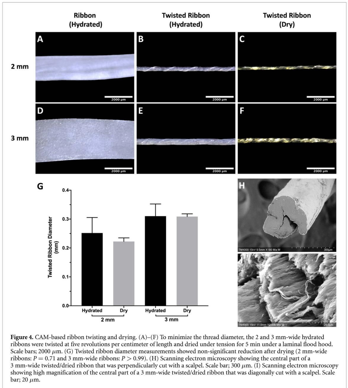
microscopy has shown that our biological thread can be cut very clearly (figure 4(H)), and high magnification imaging of diagonal cross-sections revealed the presence of stratified lamellae connected by fibrillar structures within the thread (figure 4(I)).
